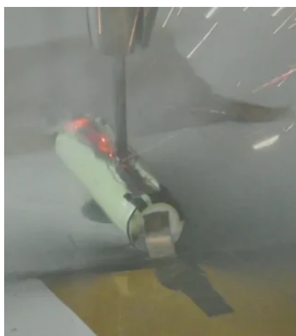
釘刺し・圧壊試験
