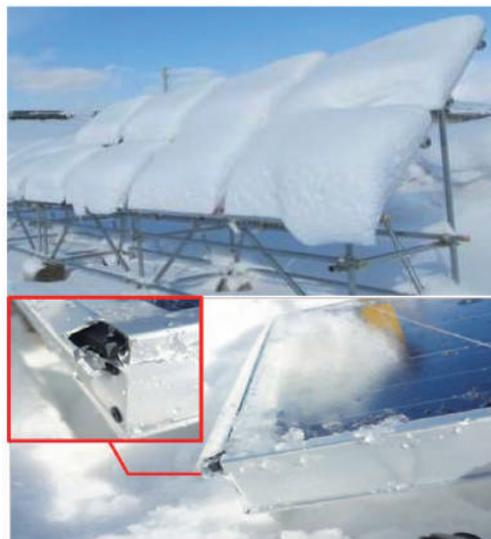
Fig. 1 Breakage of frame part due to snowfall
